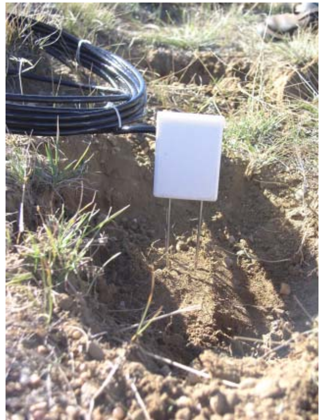
This soil moisture probe helps to predict precipitation shortages that could affect range forage production
